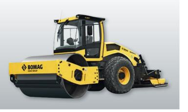
**Applications:**For compaction of soil materials like sand and gravel which tend to loosen on the surface. Also suitable for surface compaction of gravel and rubble bearing layers.
